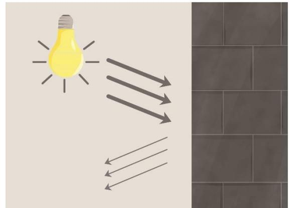
**Figure 15 Use non-reflective dark coloured surfaces.**
