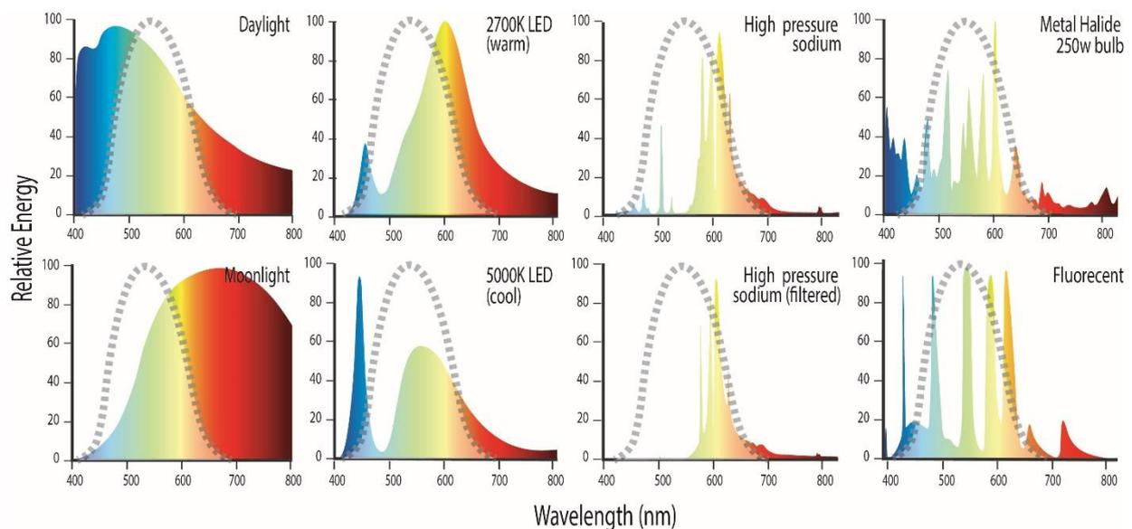
**Figure 26 Photometric instruments only quantify light that is within the CIE curve (area under grey dashed line). This is shown in comparison with the spectral curves of a range of different light sources.**
