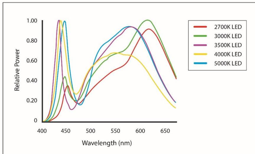
**Figure 23 Spectral curves showing the blue content of white 2700-5000 K LED lights. Note the difference in relative power output in the blue (400 - 500 nm) wavelength range. Figure courtesy of Ian Ashdown.**
