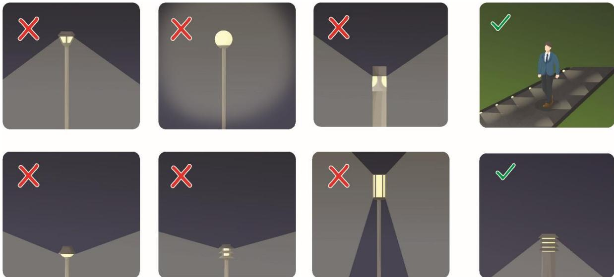
**Figure 12** Walkway lighting should be mounted as low as possible and shielded. Figure adapted from Witherington and Martin (2003)<sup>3</sup>.
