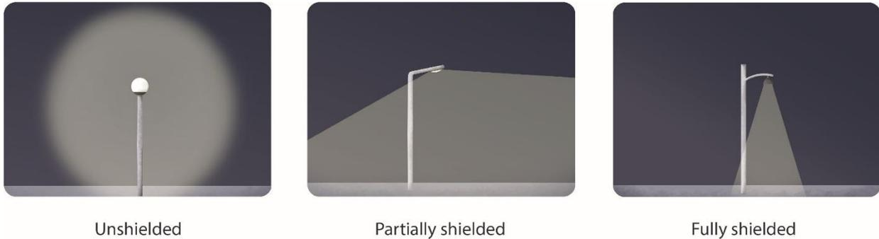
**Figure 11** Lights should be shielded to avoid lighting anything but the target area or object. Figure adapted from Witherington and Martin (2003)<sup>3</sup>.
