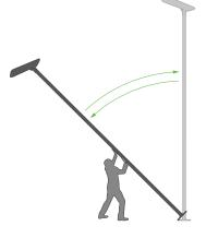
Raise/lower the lighting column and fitting safely and easily from ground level
